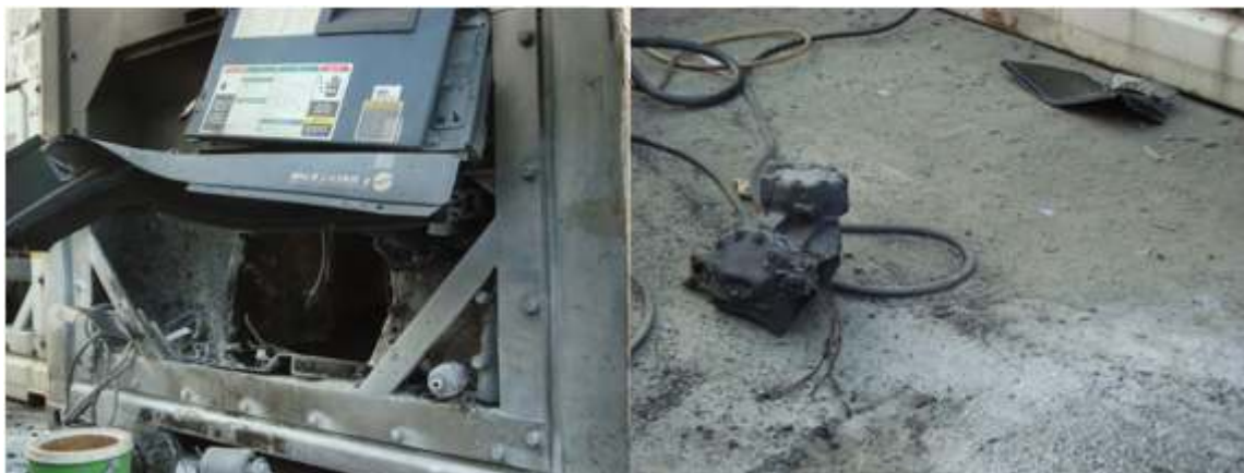
Figure 6. Refrigerated Container Destroyed by R40 Explosion with Compressor Remains
