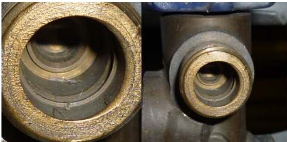
Figure 1. Uncapped Cylinder Valve (Overspray and Lint)
