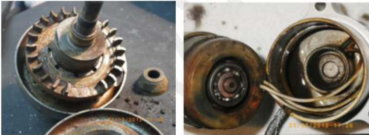
Figure 3. Contaminated Refrigerant Damage to Compressor Parts
