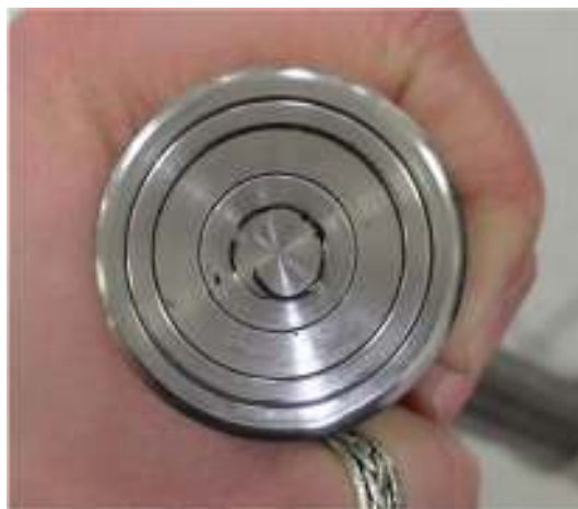
Figure 2. Mineral Oil Contamination EPDM Seal Failure
